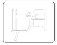
1. Open up the main frame so the seat has locked into position.
