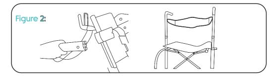
3. Insert the two rear wheels into the main frame. Make sure snap button is securely locked into your preferred position.
