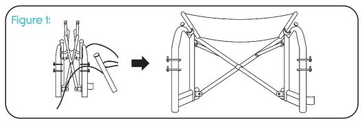
2. Insert the two height adjustable handle sections into the main frame. Make sure snap button is securely locked into your preferred position.
